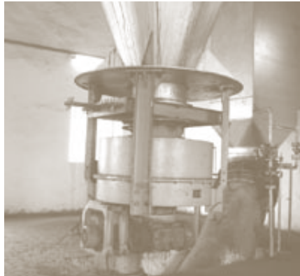
Feeding of petcoke into vertical mill by disk feeder
